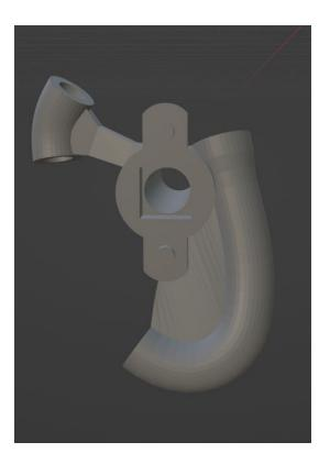
Once the cable guide has been positioned it is possible to set the cable tension before removing the je guide from the jig. With the jig still in place the guide can either be fixed to the bod of the end door panel or to a cosmetic bright polished cover plate which in turn can be fitted to the door end panel. In either case, the jig ensures correct alignment of the cable guide and, if necessary, the correct positioning of the cover plate.
